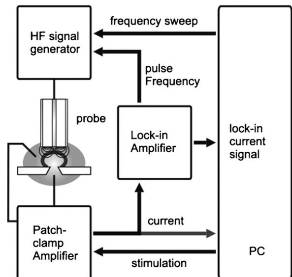
Fig. 1. Experimental setup. Patch-clamp recordings are performed with a chip-based system as described in (Bruggemann et al., 2006; Fertig et al., 2002). An open-end coaxial probe for the application of pulsed HF radiation is placed in the vicinity of the cell using a micromanipulator. The membrane current measured by a patch-clamp amplifier is fed into a lock-in amplifier and demodulated with the HF pulse frequency.
