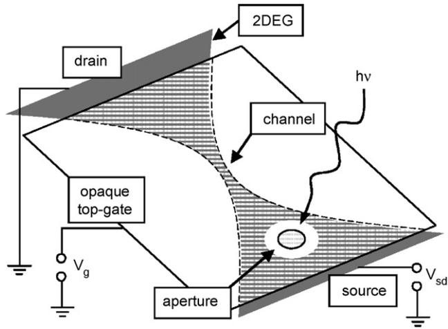
Fig. 1. Experimental circuit. A lateral constriction in a 2DEG between source and drain contacts forms a low-dimensional electron channel. The central area of the device is covered with an opaque top gate (bright rectangle). An aperture in the top gate close to the constriction defines the position where the underlying 2DEG is optically excited.
