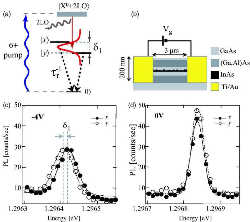
FIG. 1. (Color online) (a) Scheme of 2LO-phonon assisted quasiresonant excitation. (b) Scheme of the sample structure processed to apply an in-plane electric field. [(c) and (d)] Excitonic line measured for two different biases: (c)  $-4$  V and (d)  $0$  V for two orthogonal linear polarizations corresponding to the QD eigenstates  $|x\rangle$  and  $|y\rangle$ . Points (open and closed)—experimental data and lines (dashed and solid)—Gaussian fits.
