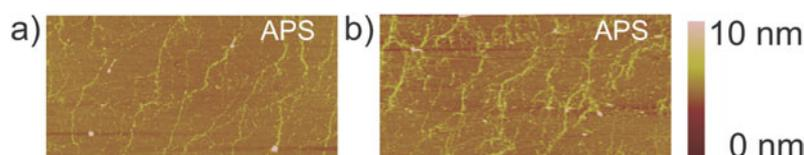
**Figure 3.** AFM images of polyaniline synthesized on DNA networks: (a) after one reaction cycle, (b) after a second application of the reaction solution to the network shown in (a). The size of the images is  $5\ \mu\text{m} \times 2.5\ \mu\text{m}$  in both cases.
