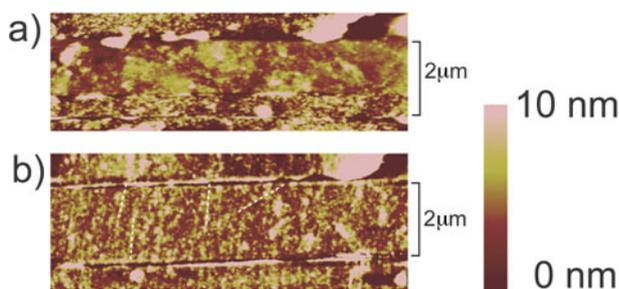
**Figure 5.** AFM images of polyaniline/DNA networks stretched between two electrodes. (a) Networks synthesized by the HRP/H<sub>2</sub>O<sub>2</sub> method, (b) synthesized by the Ru(bpy)<sub>3</sub><sup>2+</sup> method. The electrode spacing of 2 μm is indicated. The lines in (b) are drawn as a guide for the eye. The height scale is 0–20 nm.
