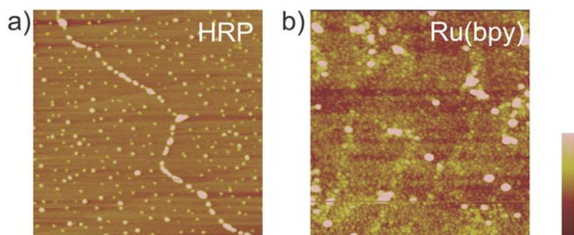
**Figure 4.** (a) AFM image of DNA/PANI synthesized by the HRP/H<sub>2</sub>O<sub>2</sub> method in solution and stretched on a mica substrate. The image size is  $2\ \mu\text{m} \times 2\ \mu\text{m}$ ; the height scale bar ranges from 0 to 5 nm. (b) DNA/PANI network synthesized by the Ru(bpy)<sub>3</sub><sup>2+</sup> method and stretched on a silicon substrate. The image size is  $1.3\ \mu\text{m} \times 1.3\ \mu\text{m}$ ; the height scale bar ranges from 0 to 10 nm.
