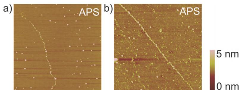
**Figure 2.** Topographic AFM images of polyaniline synthesized on DNA templates. (a) Synthesis was performed in solution, followed by stretching on mica (the image size is  $4\ \mu\text{m} \times 4\ \mu\text{m}$ ). (b) DNA templates were first combed on a silanized silicon surface, followed by polyaniline synthesis on the substrate (the image size is  $2\ \mu\text{m} \times 2\ \mu\text{m}$ ).
