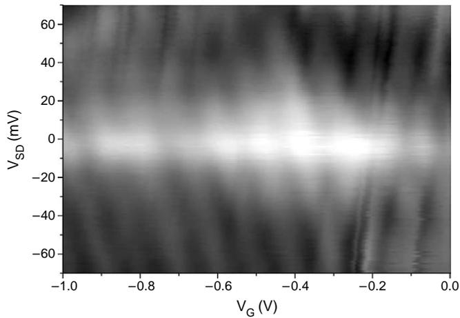
Fig. 2. Grey-scale plot of the conductance of a single multi-wall CNT as a function of back-gate voltage  $V_G$  and source–drain voltage  $V_{SD}$  at 4 K. White areas correspond to low conductance, black areas correspond to high conductance.
