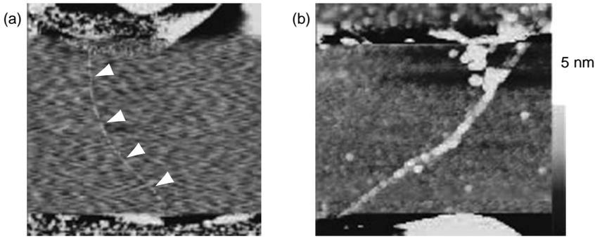
Fig. 4. Topographic AFM images of DNA stretched between two metal electrodes: (a) without and (b) with modification with Pt nanoparticles. The spacing between the electrodes is 2  $\mu\text{m}$ . In (a) the position of the DNA is indicated by white arrows.
