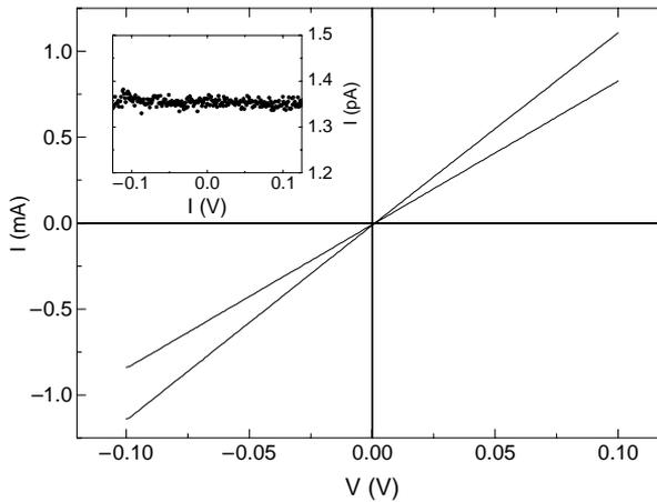
Fig. 5.  $I$ - $V$ -curves obtained from gold coated DNA molecules. The Ohmic  $I$ - $V$ -characteristics correspond to resistances of 90 and 120  $\Omega$ , respectively. In the inset, the result of a typical current-voltage measurement for unmodified DNA is displayed. From this measurement, a lower bound of 10 T $\Omega$  can be deduced for the resistance of pure  $\lambda$ -DNA.
