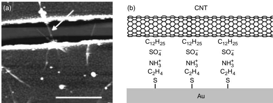
Fig. 1. (a) AFM image of two Au electrodes covered with multi-wall CNTs. The scale bar corresponds to 1  $\mu\text{m}$ . (b) Schematic representation of a CNT attached to a Au contact via cysteamine and SDS.
