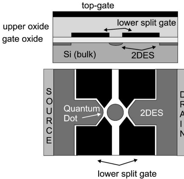
Fig. 8. Silicon quantum dot realized in bulk silicon by a dual gate technique. The positively biased metallic top-gate leads to the formation of a 2DES at the silicon/oxide interface. The split gates screen the electric fields provided by the top-gate and thus pattern the 2DES electrostatically.
