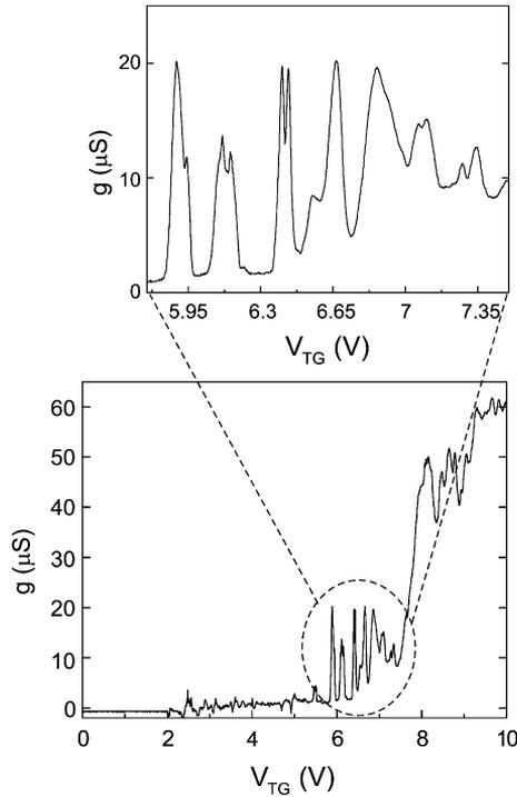
Fig. 19. Coulomb blockade oscillations in a 20 nm inversion quantum dot at a temperature of 2 K.
