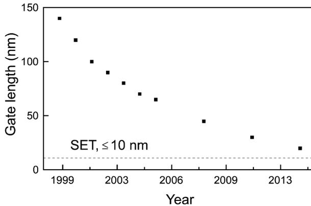
Fig. 2. Predicted gate dimensions following the SIA-roadmap. Minimal structure sizes below 10 nm necessary for reliable SET operation at room temperature are expected to become feasible in about 15–20 years.
