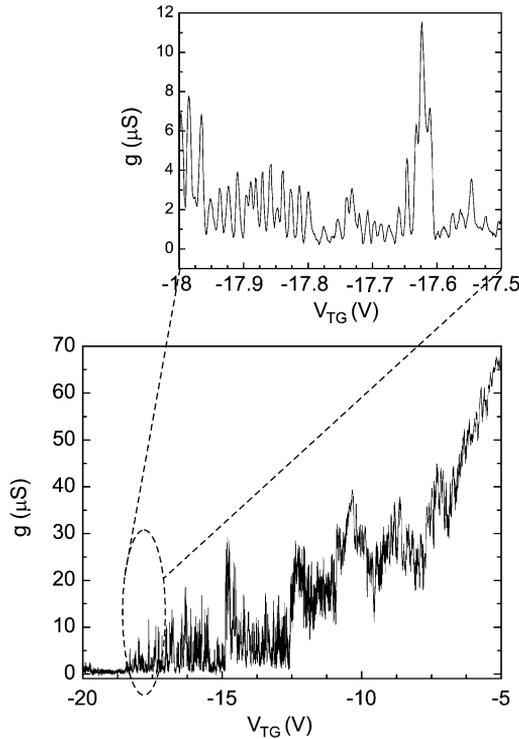
Fig. 12. Single-electron effects in a highly doped,  $10 \text{ nm}$  wide silicon wire at  $T = 2 \text{ K}$  as a function of the top-gate voltage  $V_{\text{TG}}$ . Almost periodic conductance oscillations can be found. However, both the peak amplitudes as well as the exact peak positions differ between subsequent gate sweeps.
