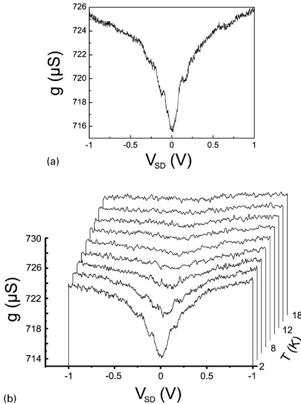
Fig. 31. (a) Conductance of a suspended quantum dot structure as a function of  $V_{SD}$ . Nonohmic behaviour is seen around  $V_{SD} = 0$  V, indicating single-electron effects. An almost periodic finestructure is superimposed. (b) Temperature dependence of the conductance. The conductance dip at zero bias vanishes with increasing temperature.
