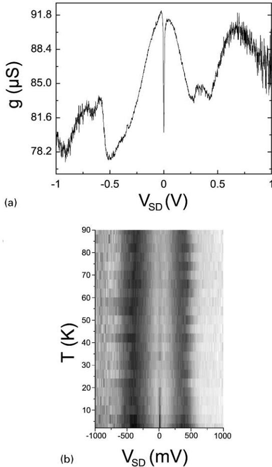
Fig. 30. (a) Conductance of the suspended nanowire at high  $V_{\text{SD}}$ . (b) A strong modulation can be seen that does not change with temperatures up to 90 K.
