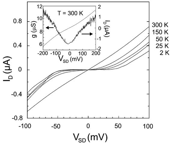
Fig. 24. Temperature dependence of the nonlinear characteristic. At  $T = 300$  K a distinct Coulomb blockade gap remains visible.
