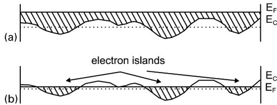
Fig. 10. Schematic drawing of the potential fluctuations along a highly doped SOI-nanowire. In (a) the highly conducting wire has a chemical potential  $E_F$  high above the fluctuating edge of the conductance band  $E_C$ . When the wire is depleted, isolated electrons islands appear, leading to a serial arrangement of SETs.
