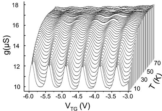
Fig. 17. Temperature dependence of the CB oscillations shown in Fig. 16(a). The oscillations remain visible up to temperatures of almost 100 K.
