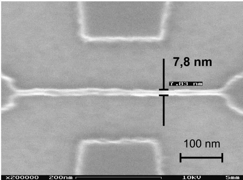
Fig. 7. Scanning electron micrograph of a 8 nm wide nanowire defined in calixarene by low-electron electron-beam lithography.
