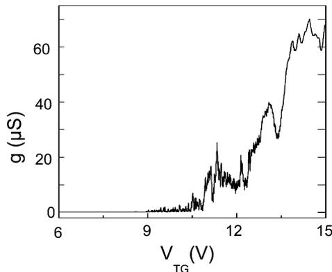
Fig. 26. Gate characteristic of a 10 nm wide, 20 nm high and 500 nm long silicon quantum wire. Electron conduction starts at a threshold voltage much higher than for similar quantum dot structures.
