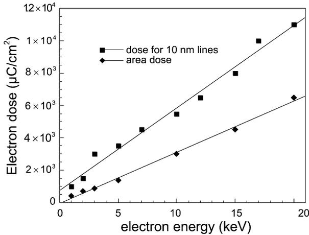
Fig. 5.  $E_1$  as a function of electron energy for narrow lines and for extended areas.  $E_1$  for narrow lines turns out to be about 1.7 times higher than for the large structures.
