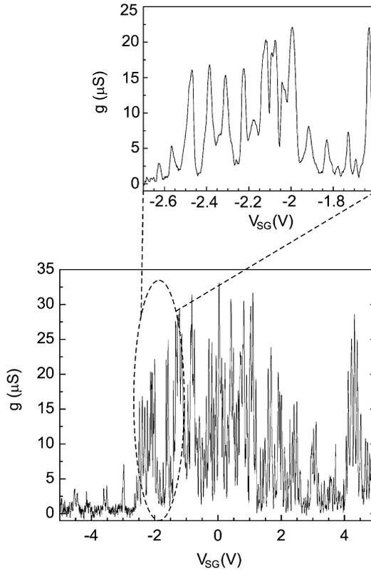
Fig. 13. Controlling the electrostatic potential of the wire via an in-plane side-gate causes conductance oscillations. The mean period of these oscillations differs from that observed in Fig. 12. The top-gate voltage in this measurement is  $V_{TG} = 17.5$  V, which allows low side-gate voltages to control the CB oscillations.
