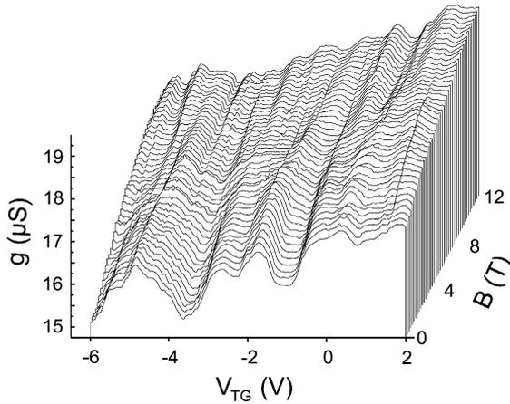
Fig. 18. CB oscillations in a quasi-metallic nanowire. No periodicity is revealed, indicating the formation of a serial arrangement of metallic islands. Although the conductance oscillations are almost unaffected by a magnetic field—indicating a hard potential wall—the tunnel junctions between adjacent electron islands in the serial arrangement show a strong influence of the magnetic field.
