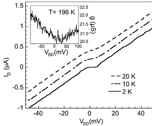
Fig. 14. Temperature dependence of the  $I_D/V_{TG}$  trace. The wire shows a distinct nonohmic behaviour at temperatures up to 20 K. Single-electron effects remain visible only weakly up to temperatures of about 200 K (see inset).
