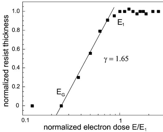
Fig. 4. Resist contrast curve for calixarene exposed with 2 keV electrons. The contrast turns out to be  $\gamma = 1.65$ .
