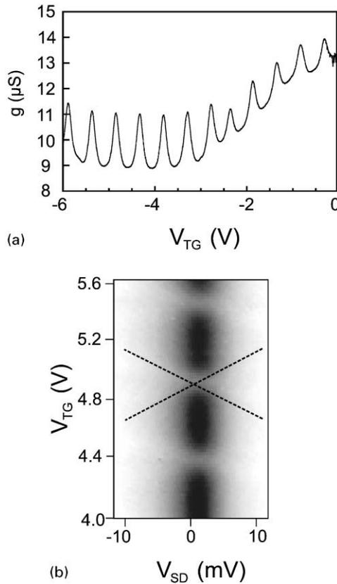
Fig. 16. (a) CB oscillations in a quasi-metallic nanowire showing almost perfect periodicity. (b) CB diamond for the structure measured in (a). From the slope of the diamond the charging energy of the dot formed inside the wire can be estimated.
