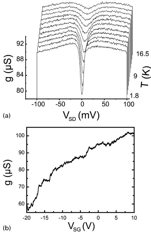
Fig. 29. (a) Temperature dependence of the conductance of a 40 nm wide and 140 nm thick suspended wire. Coulomb blockade is observed at  $V_{SD} = 0$  V. The conductance minimum remains visible up to temperatures of about 20 K. (b) Conductance as a function of  $V_{SG}$ . The nanostructure cannot be depleted fully.
