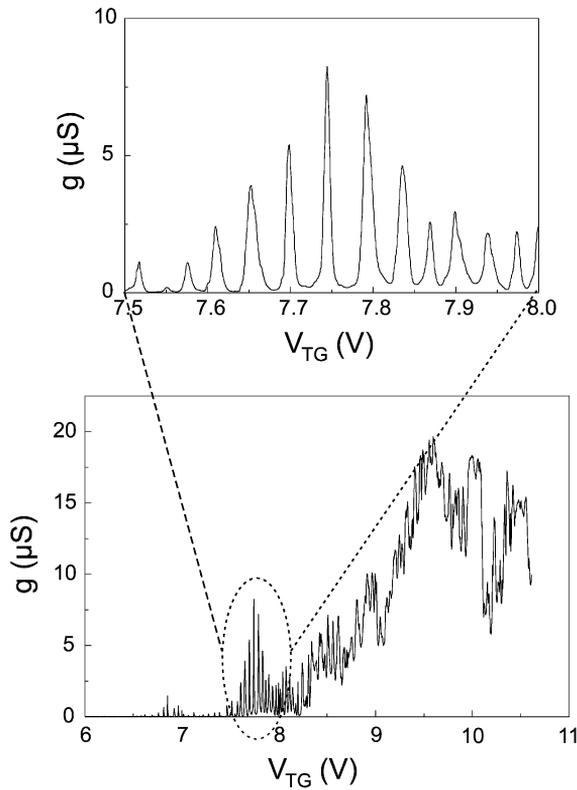
Fig. 9. Coulomb blockade oscillations of a bulk-silicon quantum dot. The charging energy is estimated to be  $E_C \approx 2$  meV.
