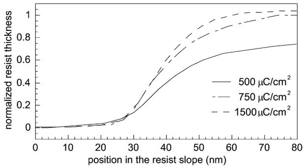
Fig. 6. Resist slope of calixarene exposed with different electron doses at an electron energy of 2 keV. For a dose of  $500 \mu\text{C}/\text{cm}^2$  below the saturation dose, the maximum resist thickness is not yet achieved.
