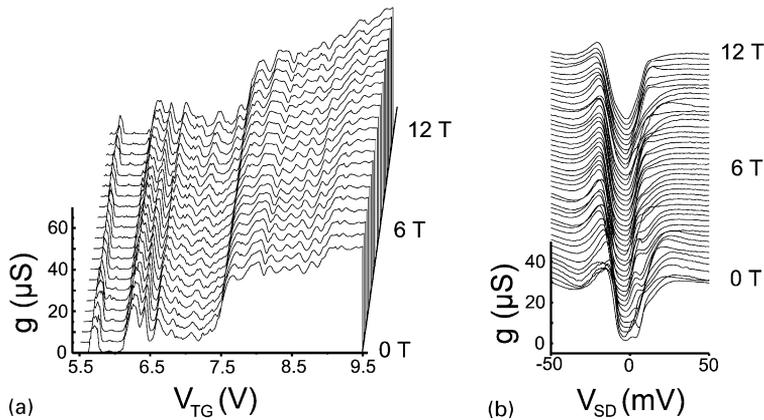
Fig. 22. Magnetic field dependence of the Coulomb blockade oscillations (a) and of the nonlinear characteristic (b) at  $T = 2$  K. No significant influence of the magnetic field can be observed.
