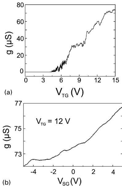
Fig. 25. (a) Gate characteristic of a 25 nm wide and 500 nm long wire. The features observed can be interpreted as electron interference effects, since no Coulomb blockade diamond could be found. (b) Conductance of a strongly inverted 25 nm wide wire as a function of  $V_{SG}$  at fixed  $V_{TG} = 12$  V.
