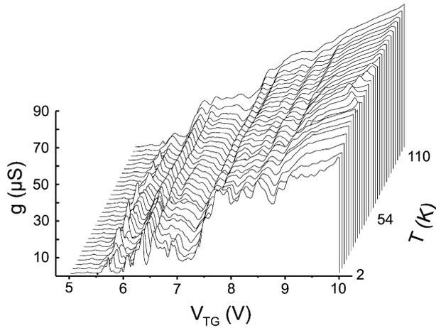
Fig. 23. Temperature dependence of the conductance oscillations of the 20 nm dot. Especially, the first conductance maximum is almost unaffected by the temperature rise up to 110 K.
