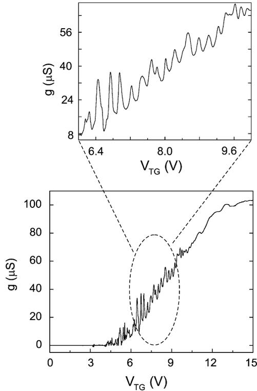
Fig. 20. Coulomb blockade oscillations in a 25 nm inversion quantum dot at a temperature of 2 K. In comparison to Fig. 19 the oscillations display a better periodicity with  $V_{TG}$ .
