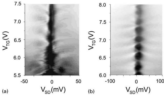
Fig. 21. Grey-scale plots of the channel differential conductances versus top-gate voltage  $V_{TG}$  and source/drain bias  $V_{SD}$  of both quantum dots are shown. From the slope of the Coulomb blockade diamonds one can determine the energy level separations. The plot in (a) (dot#1) displays a rich fine structure at nonzero bias, whereas the Coulomb blockade diamond in (b) (dot#2) almost shows a metallic behaviour.
