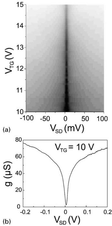
Fig. 27. Nonlinear gate characteristic of the 10 nm quantum wire in a grey-scale contour plot. No Coulomb blockade diamond is visible though a distinct conductance minimum around zero bias can be seen that decreases with increasing  $V_{TG}$ .
