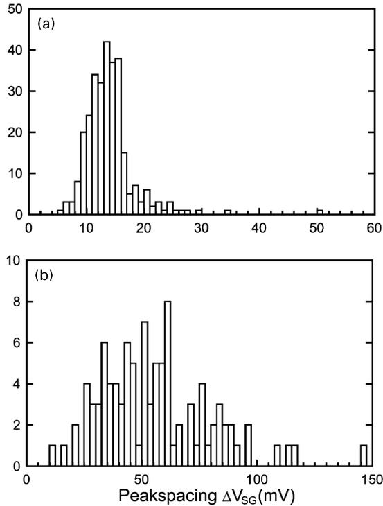
Fig. 15. Distribution for the peak-to-peak spacings found in Figs. 12 and 13. The histogram in (a) shows the distribution for  $V_{TG}$ , in (b) the curve for  $V_{SG}$  is shown. The curve in (b) clearly shows a larger broadening than the plot in (a). The normalized standard deviation for the distribution in (a) is  $\sigma_{TG} = 0.32$  and in (b)  $\sigma_{SG} = 0.43$ .
