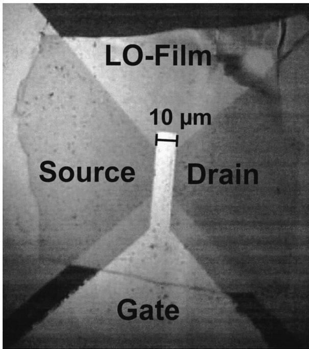
FIG. 3. Micrograph of the realized LO-MOSFET: Pt pads were used for source and drain contacts. The LO film was laterally patterned in order to form a mesa structure in the active region for device isolation.
