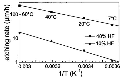
FIG. 2. Temperature dependence of the underetching rate in 48% HF and 10% HF. The common Arrhenius-type plot and no significant deviations from the vertical etching rates are found.
