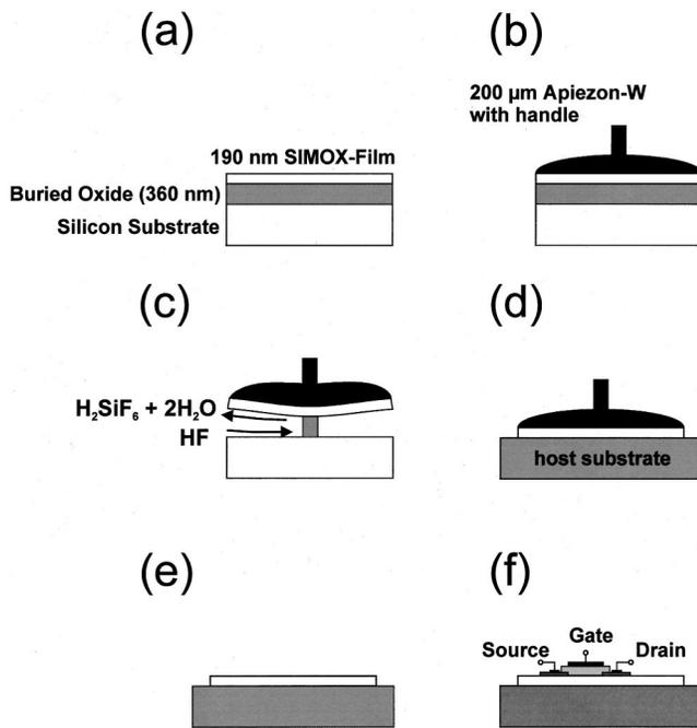
FIG. 1. Schematically shown is the process of fabricating silicon LO films: Starting from a slightly boron-doped silicon-on-insulator structure (a), the silicon film is covered by a thick Apiezon-W film protecting the surface (b) and subsequently underetched in diluted HF (c) and attached onto an arbitrary substrate by van der Waals forces (d). The Apiezon-W is removed (e) and an enhancement MOSFET is defined (f).
