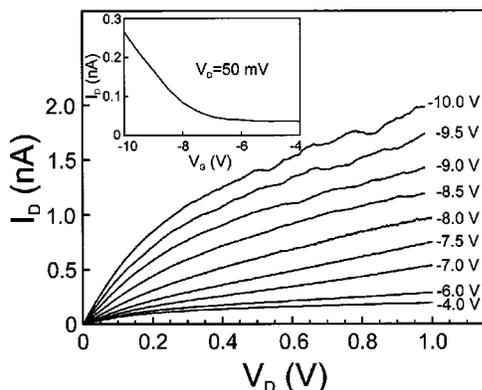
FIG. 4. Output characteristic  $I_D$  vs  $V_D$  at fixed gate voltages and transfer characteristic [ $I_D$  vs  $V_G$  (inset)] for the silicon thin-film  $p$ -channel LO-MOSFET ( $T = 300 \text{ K}$ ).
