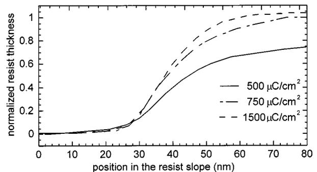
Fig. 3. Resist slope for electron doses of 500, 750, and  $1500 \mu\text{C}/\text{cm}^2$ . Although the maximum resist thickness is almost achieved at  $E=750 \mu\text{C}/\text{cm}^2$ , the slope still gets steeper for higher electron doses.
