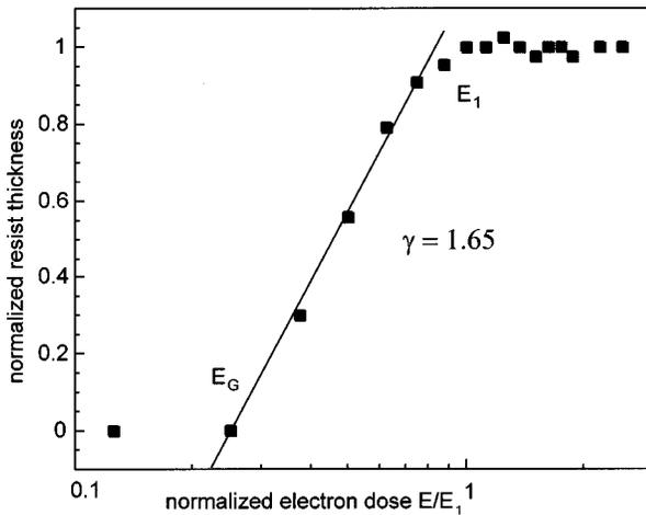
Fig. 1. Resist contrast curve for exposure at an electron energy of 2 keV. The minimum gel dose is  $E_G=200 \mu\text{C}/\text{cm}^2$ , and the saturation or maximum dose is  $E_1=800 \mu\text{C}/\text{cm}^2$ . The contrast  $\gamma$  is measured to be  $\gamma=1.65$ .
