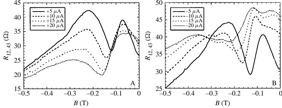
**Fig. 2.** Four-terminal bend resistance  $R_{12,43}$  for high positive (a) and negative (b) dc currents.
