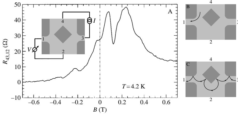
**Fig. 1.** A, Four-terminal bend resistance  $R_{43,12}$  of a cross-junction with a symmetry-breaking scatterer. The inset is an atomic force micrograph of the device. B and C, Typical electron trajectories at positive magnetic fields.
