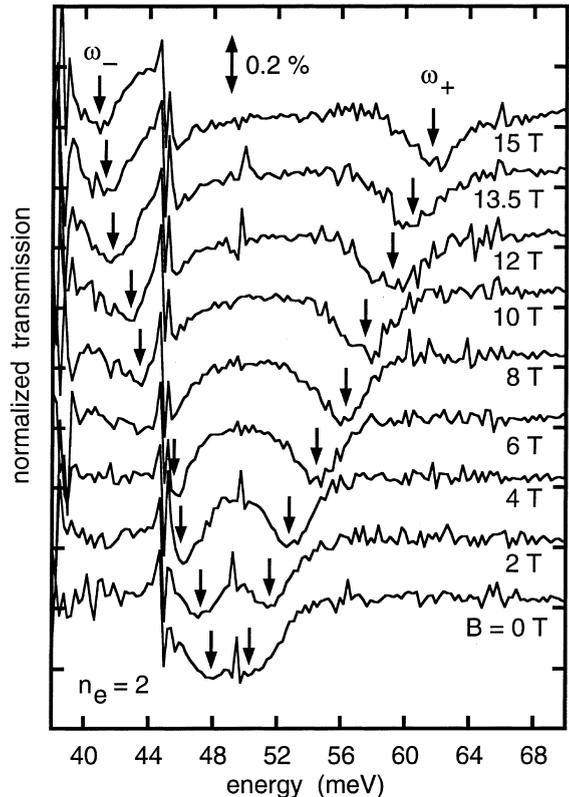
Fig. 3. FIR spectra of self-organized dots (occupied with  $n_e \approx 2$  electrons each) for different magnetic fields. The well-known, two-mode spectrum of parabolically confined quantum dots is observed. Curves are offset for clarity.
