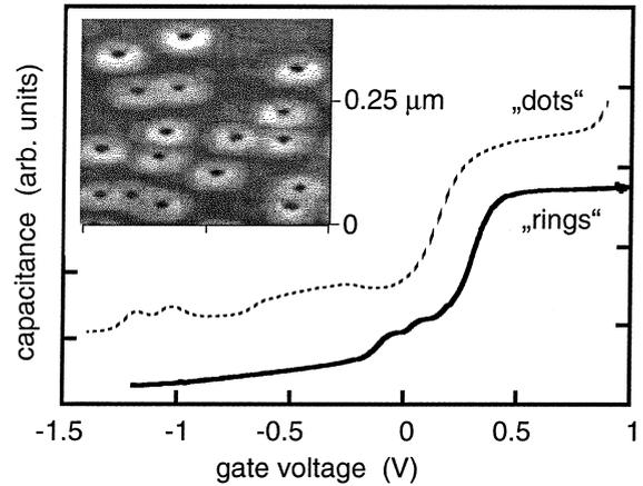
Fig. 6. Charging characteristic of self-organized ‘rings’, compared to the CV spectrum of conventional dots. The inset displays an atomic force micrograph of the uncovered ring structures.
