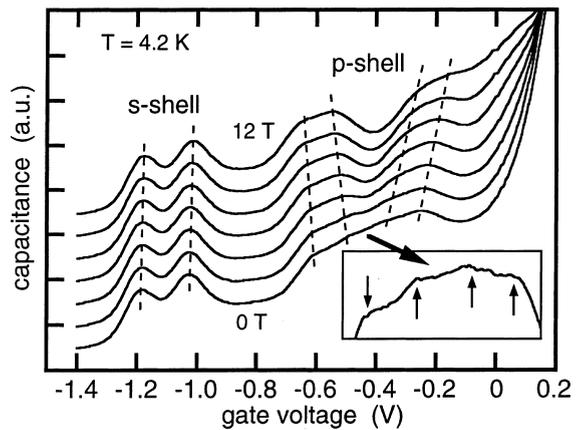
Fig. 2. Charging spectra of self-organized InAs quantum dots. Individual charging peaks are resolved for both s- and p-shells (see also inset). From bottom to top curve, the magnetic field is increased from 0 to 12 T in steps of 2 T, and the orbital Zeeman splitting of the p-shell is clearly observed. Curves are offset for clarity.
