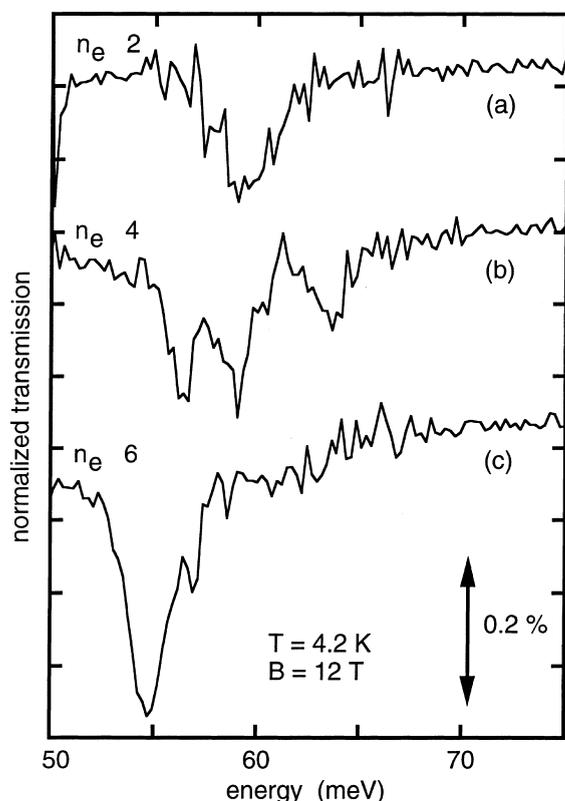
Fig. 4. FIR excitation spectra at  $B = 12$  T for different occupation numbers  $n_e$ . For a partly occupied p-shell ( $n_e = 4$ ), a splitting of the  $\omega_+$ -mode into three resonances is observed.
