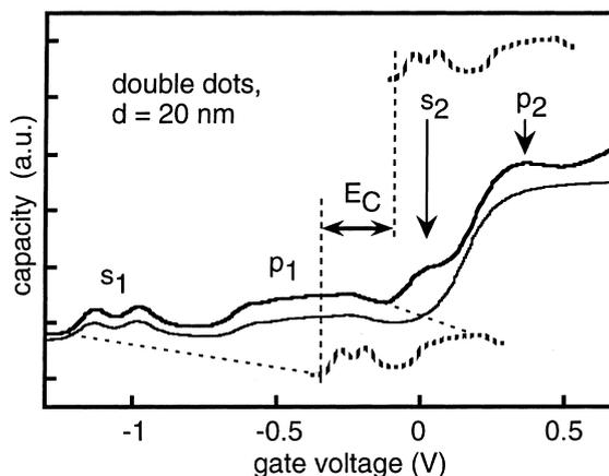
Fig. 5. CV spectrum of a double-dot-layer sample (thick solid line) compared to that of a single-layer structure (thin solid line). In the double-layer sample, two additional structures are observed (arrows), which are attributed to the charging of the second dot layer.
