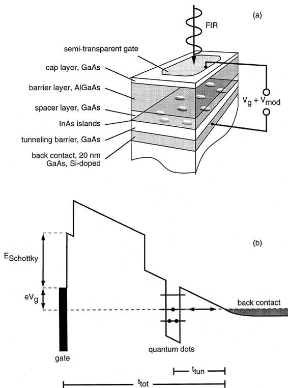
Fig. 1. (a) Schematic of the measurement geometry and layer sequence of the field-effect transistor structure with the embedded InAs quantum dots. (b) Sketch of the conduction band edge of the device. For details, see text.
