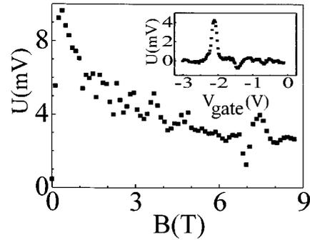
FIG. 2. The amplitude of the signal  $U$  as a function of the magnetic field  $B$ . The insert shows the amplitude of the signal  $U$  as a function of the gate voltage  $V_{\text{gate}}$  at  $B=4.16$  T.
