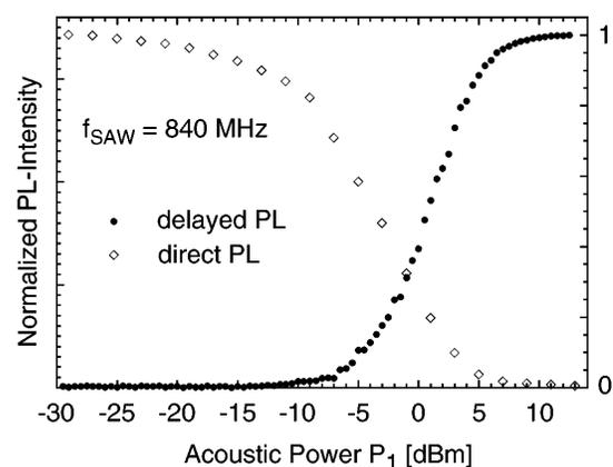
FIG. 3. Normalized direct and delayed PL intensities as a function of the acoustic power  $P_1$ . Efficient ambipolar transport of charges resulting in a time-delayed PL signal requires a minimum threshold acoustic power of  $P_1 = -5$  dBm which corresponds to a minimum lateral electric field strength ( $E_l = 2$  kV/cm). This threshold coincides with the quenching of the direct PL signal.
