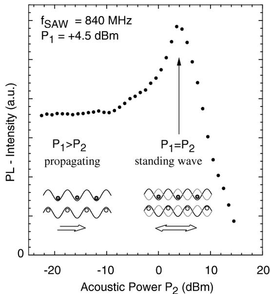
FIG. 4. Direct PL intensity at  $x = x_c$  as a function of the acoustic power  $P_2$  for a constant acoustic power  $P_1 = 4.5$  dBm. For the standing wave geometry at  $P_1 = P_2$  the spatial separation between electrons and holes is lifted, resulting in a recovered PL intensity due to the increased transition probability.
