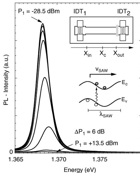
FIG. 1. Photoluminescence spectra of a single 10 nm wide InGaAs/GaAs quantum well structure for different acoustic powers. The optical excitation occurs at the site  $x = x_c$  with an intensity of  $10 \text{ mW/cm}^2$  and wavelength  $\lambda_{\text{laser}} = 780 \text{ nm}$ . The insets schematically depict the sample design with two interdigital transducers and the storage of optically generated excitons in the potential of a surface acoustic wave.
