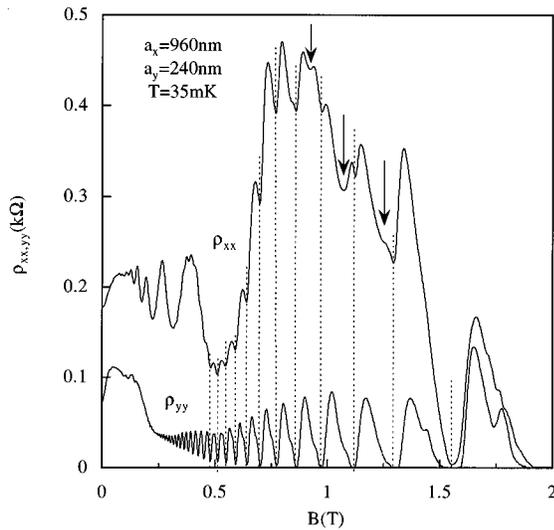
FIG. 4. Magnetoresistance for a rectangular lattice with an anisotropy of  $a_x:a_y=960\text{ nm}:240\text{ nm}=4:1$ . The superimposed SdH oscillations in  $\rho_{yy}$  are periodic in  $1/B$  while in  $\rho_{xx}$  additional oscillations arise (see arrows).
