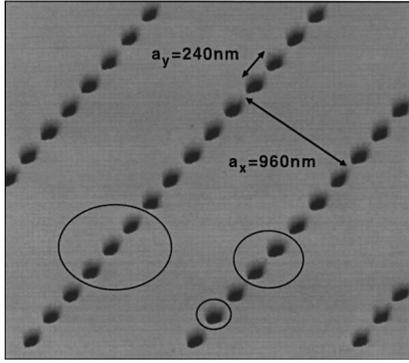
FIG. 1. Image of a wet etched surface of a GaAs/Al<sub>x</sub>Ga<sub>1-x</sub>As heterostructure. The rectangular antidot pattern with lattice periods  $a_x = 960$  nm and  $a_y = 240$  nm was produced by electron beam lithography. The image is taken with an atomic force microscope. If a magnetic field is applied perpendicular to the plane of the 2DEG the electrons travel around groups of antidots as it is schematically shown in the figure.
