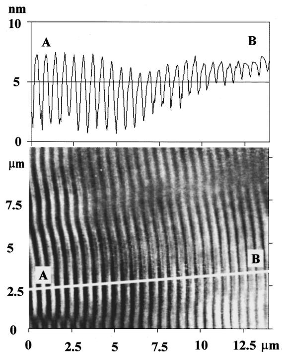
FIG. 5. AFM topography of the surface grating (lower part). Surface profile along the section A, B (upper part). Periodicity of 522 nm and height amplitudes between 3 and 5 nm are found.
