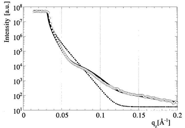
FIG. 4. Specular intensity ( $m=0$ ) as a function of perpendicular momentum transfer  $q_z$ . Open circles represent the experimental data, the dashed line is a calculation using a Gaussian surface roughness of 2.3 nm. The solid line shows the result of a fit for which the surface grating has been replaced by a sinusoidal surface layer with an average thickness of 6 nm.
