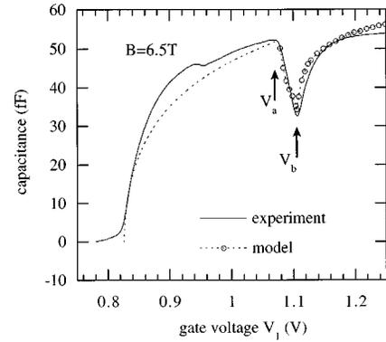
FIG. 2. The full line presents the differential capacitance of a sample recorded as function of the gate voltage  $V_1$  at  $\Delta V = 3.2$  V and a magnetic field of  $B = 6.5$  T. The dashed line is calculated according to a model described in the text.
