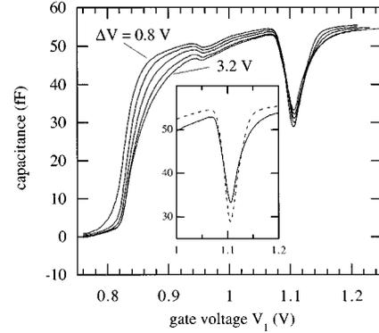
FIG. 3. Capacitance traces of the same device as in Fig. 2 recorded at different voltage differences  $\Delta V$  between center gate and side gates. The bottom trace is recorded at  $\Delta V = 3.2$  V and the difference is decreased in steps of 0.6 V. The inset depicts the behavior at filling factor  $\nu = 2$  for  $\Delta V = 3.2$  V (full line) and 0.8 V (dashed line), respectively.
