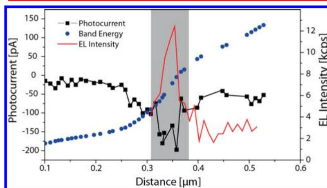
**Figure 5.** Spatial correlation between EL and photocurrent. Antenna-enhanced zero bias photocurrent measured along the device (black square symbols), band energy (blue round symbols) and measured EL intensity (red line). The EL peaks at the position of highest photocurrent and highest band energy gradient.
