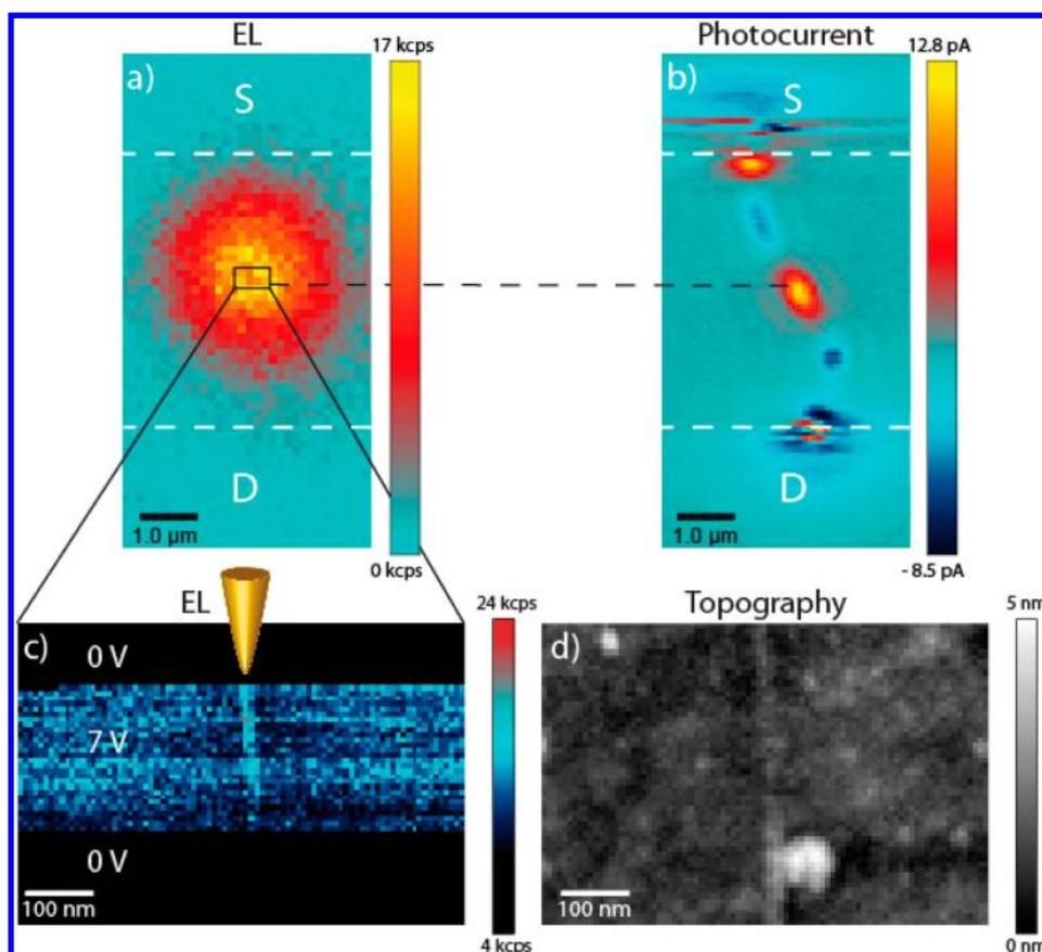
**Figure 6.** Antenna-enhanced EL of a second device. (a) Confocal EL image and (b) confocal photocurrent image. The EL occurs at the position of strongest photocurrent signal. (c) Antenna-enhanced EL image. The confocal and antenna-enhanced EL appear upon biasing (7 V). (d) Simultaneously taken topography image. The high spatial resolution reveals an emitting nanotube segment that is longer than 100 nm.
