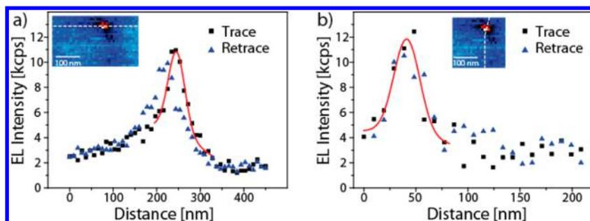
**Figure 4.** Size of the source of electroluminescence. (a) Antenna-enhanced EL cross sections perpendicular and (b) along the CNT. The red lines are a guide to the eye to highlight the near-field contribution. Because the cross section taken along and perpendicular to the CNT have about the same width of about 40 nm the extension of the EL source along the CNT needs to be substantially smaller, probably below 20 nm.
