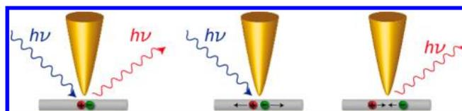
**Figure 1.** Applications of antenna enhancement. (a) Optical spectroscopy, (b) photovoltaics, and (c) electroluminescence (adapted with permission from ref 3. Copyright OSA 2009).
