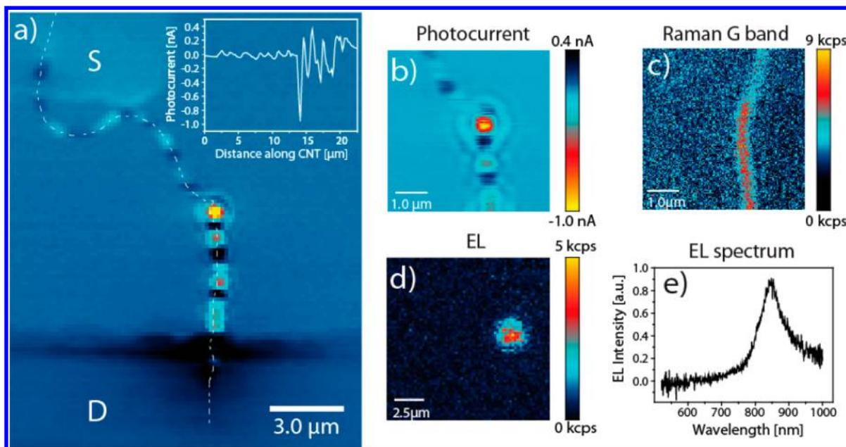
**Figure 2.** Confocal study. (a) Confocal zero bias photocurrent image of a CNT network on glass. S and D denote source and drain electrode. The inset shows the zero bias photocurrent signal detected along the white dashed line. (b) Confocal zero bias photocurrent image (zoom). (c) Simultaneously taken confocal Raman G band image of the same region as in (b). (d) Confocal electroluminescence image. (e) Electroluminescence spectrum recorded at the bright EL spot in (d).
