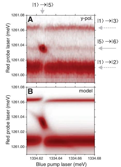
**Fig. 4.** Two-laser experiment showing conditional interaction in a CQD. Gate voltage is fixed at 130 mV, with  $y$ -polarized red and blue lasers. **(A)** Absorption of red probe laser in the presence of a strong (undetected) blue pump laser shows a conditional shift of the red QD transition energy when the blue laser is resonant with the  $X_b^-$  transition (vertical arrow). **(B)** Calculated absorption for the experiment depicted in (A).
