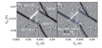
FIG. 3. (Color online) (a) Charge stability diagram as in Fig. 2 ( $V_{\rm DQD}$  =  $-241.1\,\mu\rm V$ ) but with overall reduced and asymmetric tunnel couplings. The tunnel barrier between the double QD and the drain lead is larger than the other tunnel barriers. Distinct kinks in the black charging lines are reminiscent of the bias triangles and can be used for determining the conversion factors. (b) Same data as in (a); reconstruction of the bias triangles (solid lines).
