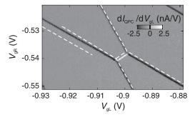
FIG. 6. The grayscale plot shows the zero-bias data from Fig. 4(a), with the charging lines from Fig. 4(b) ( $V_{\rm DQD}=-387.5~\mu{\rm V}$ ) superimposed as dashed lines
