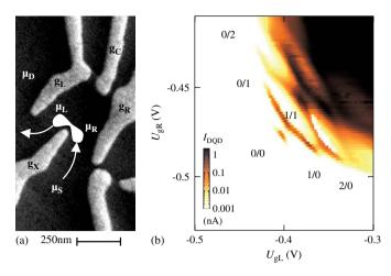
Fig. 1. (a) SEM micrograph of the gate electrode geometry used to define a DQD. The approximate position of the DQD and the current path is indicated in white. (b) Current through the DQD as function of the side gate voltages  $U_{\rm gL}$  and  $U_{\rm gR}$  ( $U_{\rm SD,DC}=50\,\mu\rm V$ , logarithmic color scale).
