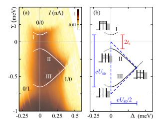
FIG. 2: (Color online) (a) Measurement of SET current through a one–electron DQD at  $U_{\rm SD}=-0.75\,\mathrm{mV}$  and  $U_{\rm gC}=-1.47\,\mathrm{V}$  (logarithmic scale), including model lines for strong interdot coupling (see (b)). (b) Corresponding model expectations for SET transport features at finite source–drain bias in the two cases of weak (dashed lines) versus strong (solid and dotted lines) interdot coupling.
