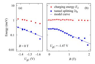
FIG. 4: (Color online) (a) Tunnel splitting  $2t_0$  of the one-electron DQD and charging energy for the second electron  $E_2$  in dependence on gate voltage  $U_{\rm gC}$ . (b)  $E_2$  and  $2t_0$  plotted as function of a perpendicular magnetic field.
