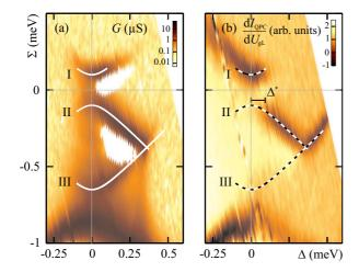
FIG. 3: (Color online) (a) Differential conductance  $dI_{\rm DQD}/dU_{\rm SD}$  through the DQD corresponding to the current measurement shown in Fig. 2(a) (identical parameters, logarithmic scale). (b) Corresponding differential transconductance  $dI_{\rm QPC}/dU_{\rm gL}$  through a nearby QPC (linear scale). For both plots, the model lines are identical to those in Fig. 2.
