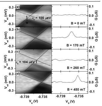
FIG. 3. Transport spectrum for (a) B=0, (b) 170, (c) 260, and (d) 450 mT. The line plots give the conductance near zero bias. At certain magnetic fields (b),(d) excited quantum dot states with higher magnetic momentum are brought into resonance with the cavity phonon reenabling single electron tunneling. Otherwise (a),(c) transport is suppressed due to phonon blockade with an excitation barrier of around 100  $\mu eV$ .
