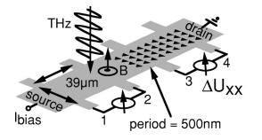
FIG. 1. Sample layout and setup for photoconductivity measurements.
