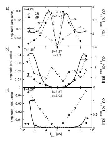
FIG. 4. Amplitudes of cyclotron resonance (open circles) and magnetoplasmon (solid dots) photoresponse in comparison to the longitudinal resistance  $dU_{xx}/dI_{bias}$  as a function of the bias current applied between source and drain.
