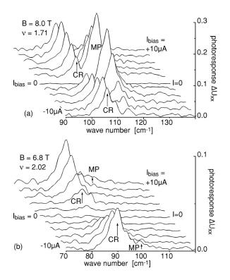
FIG. 3. Photoconductivity spectra at a magnetic field (filling factor) of (a) B=8 T ( $\nu=1.7$ ) and (b) B=6.8 T ( $\nu=2$ ) for different bias currents ranging from  $I=-10 \ \mu$ A to  $+10 \ \mu$ A.
