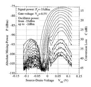
FIG. 2. The intermediate frequency power level is plotted as a function of the applied source-drain bias for different local oscillator power levels (-35 dB m to - 2 dB m - corresponding to the lowest and the highest trace) at fixed gate voltage. The signal power level is fixed at -35 dB m, the temperature of the sample is 4.2 K.
