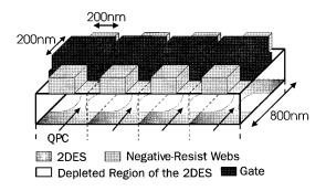
FIG. 1. The parallel device geometry used in these experiments is schematically illustrated. The Schottky gate height is periodically modulated via the insulating resist strips defined on the surface of the semiconductor using high-resolution electron-beam lithography.
