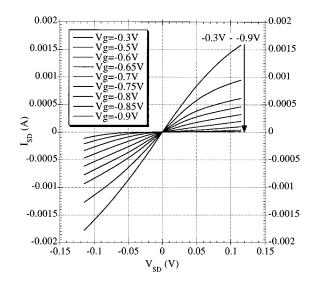
FIG. 3. Current-voltage-characteristics for different gate voltages under microwave bias are shown for the relevant voltage-region from -0.3 up to -0.9 V.
