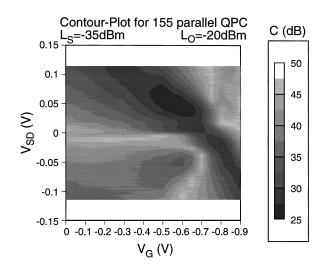
FIG. 4. A summary of the conversion-loss data is shown in a contour plot as a function of the applied source drain and gate voltages. The results shown are for the device with 155 QPCs.
