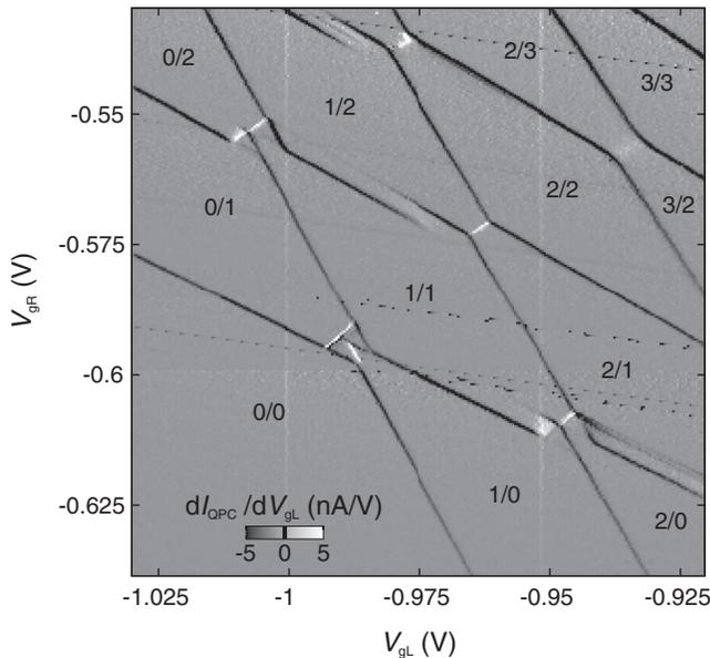
FIG. 5. Larger section of the charge stability diagram for an asymmetrically tunnel coupled double QD similar to that of Fig. 4(b) at  $V_{DQD} = -387.5 \mu\text{V}$ . Absolute values of the electron numbers in the left ( $L$ ) and right QD ( $R$ ) are given as  $L/R$ . Barely visible almost horizontal lines are related to resonances in the detector QPC.
