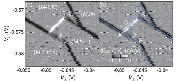
FIG. 3. (Color online) (a) Charge stability diagram as in Fig. 2 ( $V_{\text{DQD}} = -241.1 \mu\text{V}$ ) but with overall reduced and asymmetric tunnel couplings. The tunnel barrier between the double QD and the drain lead is larger than the other tunnel barriers. Distinct kinks in the black charging lines are reminiscent of the bias triangles and can be used for determining the conversion factors. (b) Same data as in (a); reconstruction of the bias triangles (solid lines).
