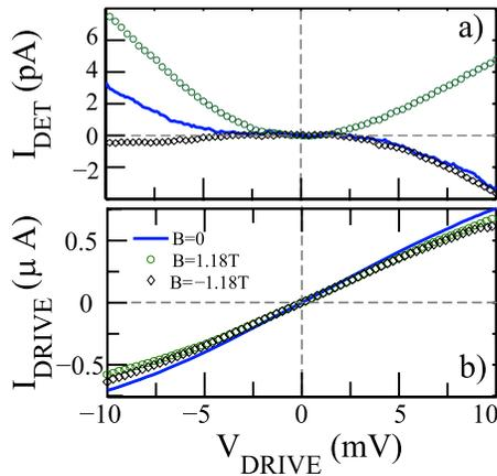
FIG. 2. (Color online) Results for sample 1 at 4.2 K. (a) Detector current at  $B=0$  (solid line) and in moderate magnetic fields (symbols, same legend as in panel b) as a function of drive bias. (b)  $I$ - $V$  curves of the drive QPC taken simultaneously with the data in (a).
