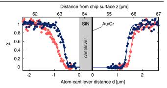
FIG. 2 (color online). Fraction  $\chi$  of atoms remaining in the trap after  $t_h=1$  ms at distance d from the cantilever surface. Blue (red) data points correspond to a trap with  $\omega_z/2\pi=10.0$  kHz (5.1 kHz). Solid lines: fit with a simple model [11,19]. The extracted cantilever position is shown.
