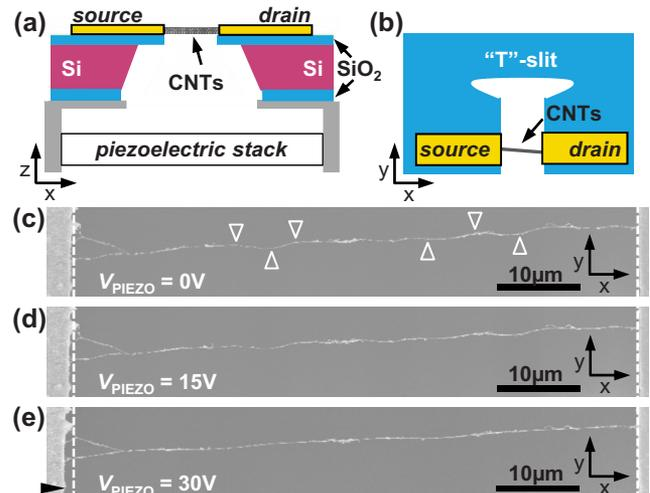
FIG. 1. (Color online) Schematic side (a) and top (b) view of a Si/ $\text{SiO}_2$  sample with a "T"-slit and freely suspended single-walled CNTs mounted on a piezoelectric stack. Applying a voltage  $V_{\text{PIEZO}}$  to the piezoelectric stack allows applying uniaxial strain to the CNTs. [(c)–(e)] SEM images of CNTs at  $V_{\text{PIEZO}}=0, 15,$  and  $30$  V at RT.
