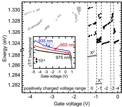
FIG. 2. (Color online) All observed resonance peak positions are plotted as a function of gate voltage. The charging events of the QD can be seen as jumps in energy and are marked by dashed lines. The charge states are listed. The inset shows the QD independent background signal for three laser wavelengths and the circle marks the QD resonances on top of this background.
