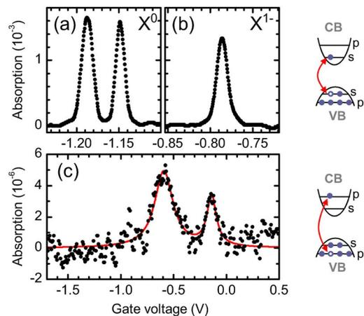
FIG. 1. (Color online) (a)  $s$ - $s$  transmission spectrum of an uncharged QD as sketched on the right side. (b) spectrum of an  $s$ - $s$  transition on the same QD charged with one electron. (c)  $p$ - $p$  transitions as sketched on the lower right. The three resonances differ in charge. All data were taken under an intensity of 16 nW. The integration time per data point is 1 s for (a) and (b), and 20 s for (c).
