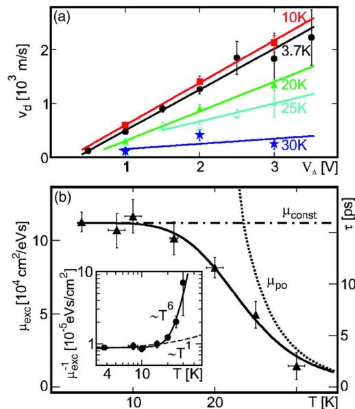
FIG. 3. (Color online) (a) Measured excitonic drift velocity  $v_d$  vs the voltage drop  $V_d$  at various bath temperatures  $T$ . The differential mobility is obtained from linear curves fitted to the data. (b) Excitonic mobility  $\mu_{exc}$  and scattering time  $\tau$  (right vertical axis) as a function of the temperature. Inset: Double logarithmic representation of the inverse mobility  $1/\mu_{exc}$  vs temperature. The solid lines are theoretical fits to the data.
