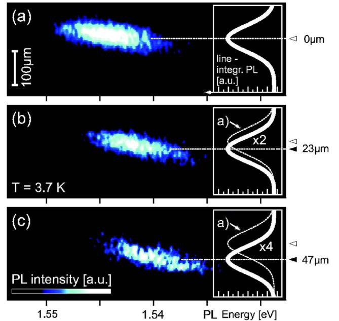
FIG. 2. (Color online) Photoluminescence images showing drift of excitons at  $T=3.7 \text{ K}$ , taken at (a)  $t=0 \text{ ns}$ , (b)  $t=20 \text{ ns}$ , and (c)  $t=40 \text{ ns}$  after enabling the excitonic gradient potential. Insets: Energy-integrated representations of the data (solid curves). In the insets of (b) and (c) the lateral PL distribution of the cloud at  $t=0 \text{ ns}$  is shown as a dashed curve.
