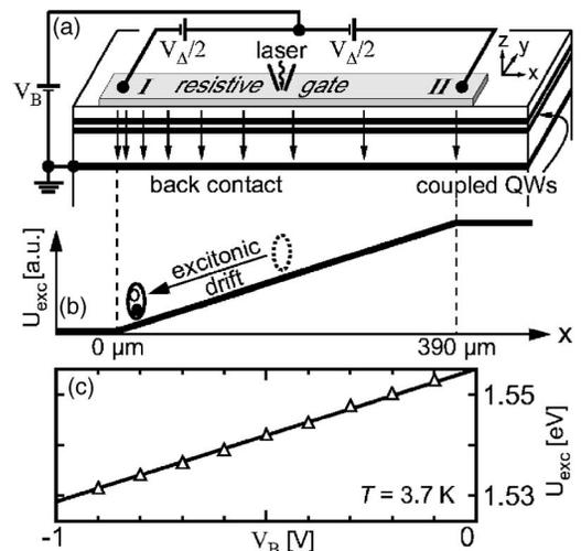
FIG. 1. (a) Excitonic time-of-flight apparatus. A current-carrying top gate (gray) defines a laterally varying vertical electric field (vertical arrows). (b) Sketch of the in-plane excitonic potential between contacts “I” and “II” due to the quantum confined Stark effect (QCSE). The slope of the gradient is tunable via the voltage  $V_\Delta$ . (c) Calibration of the QCSE shift by application of a dc voltage  $V_B$  to the top gate.
