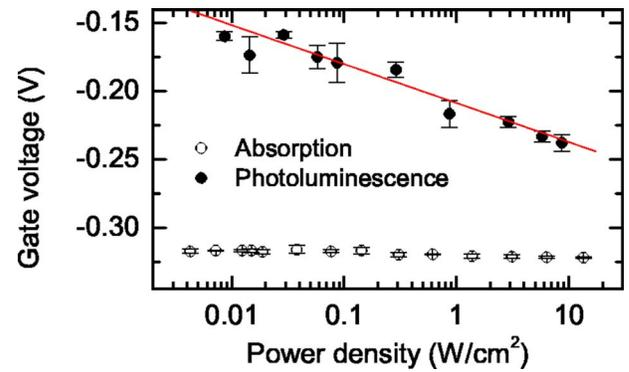
FIG. 3. (Color online) Resonant gate voltage against pump power density for PL and absorption spectroscopy, in both cases keeping the wavelength constant. The data were taken from two different QDs at  $4.2 \text{ K}$  and represent typical behavior for the QDs embedded in the heterostructure of Fig. 1. The line describing the PL data is a guide to the eye.
