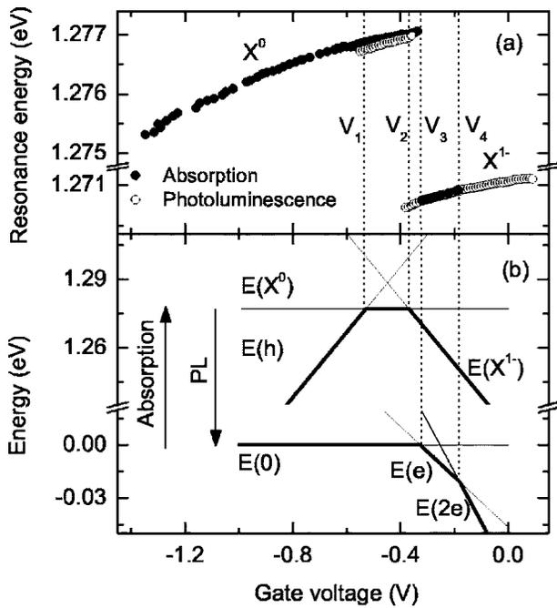
FIG. 4. (a) Behavior of the PL and absorption energies as a function of gate voltage,  $V_g$ . The PL energies are corrected for space charge effects as described in the text. (b) Energy of the 0, e, 2e, h,  $X^0$  and  $X^{1-}$  states as a function of  $V_g$ . The bold lines show the energetically favored states with (upper part) and without (lower part) a hole.
