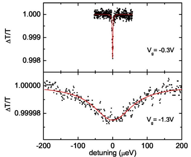
FIG. 5. (Color online) Absorption in two different gate voltage regions. The upper graph shows the absorption resonance at a gate voltage of  $-0.3 \text{ V}$  where the linewidth is not influenced by tunneling and the lower graph shows the resonance at  $-1.3 \text{ V}$  where the linewidth is completely dominated by tunneling. The solid lines are Lorentzian fits to the data with linewidths  $2.25 \mu\text{eV}$  at  $V_g = -0.3 \text{ V}$  and  $136 \mu\text{eV}$  at  $V_g = -1.3 \text{ V}$ .
