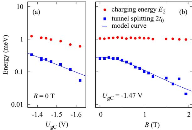
FIG. 4: (Color online) (a) Tunnel splitting  $2t_0$  of the one-electron DQD and charging energy for the second electron  $E_2$  in dependence on gate voltage  $U_{gC}$ . (b)  $E_2$  and  $2t_0$  plotted as function of a perpendicular magnetic field.
