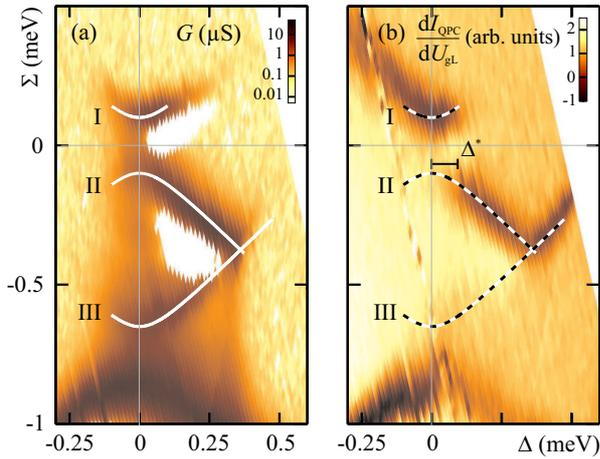
FIG. 3: (Color online) (a) Differential conductance  $dI_{DQD}/dU_{SD}$  through the DQD corresponding to the current measurement shown in Fig. 2(a) (identical parameters, logarithmic scale). (b) Corresponding differential transconductance  $dI_{QPC}/dU_{gL}$  through a nearby QPC (linear scale). For both plots, the model lines are identical to those in Fig. 2.
