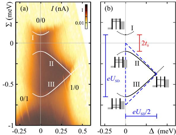
FIG. 2: (Color online) (a) Measurement of SET current through a one-electron DQD at  $U_{SD} = -0.75$  mV and  $U_{gC} = -1.47$  V (logarithmic scale), including model lines for strong interdot coupling (see (b)). (b) Corresponding model expectations for SET transport features at finite source-drain bias in the two cases of weak (dashed lines) versus strong (solid and dotted lines) interdot coupling.
