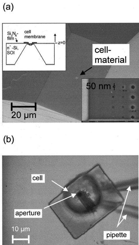
FIG. 1. (a) SEM micrograph of a V-groove in (100) silicon with a suspended  $\text{Si}_3\text{N}_4$  layer on top. In the central aperture cell material is incorporated. The upper inset depicts the arrangement of the semiconductor-cell hybrid. The lower inset shows a series of holes in a suspended membrane with dimensions down to 50 nm. (b) Photograph of the probe with the cell positioned on top of the aperture.
