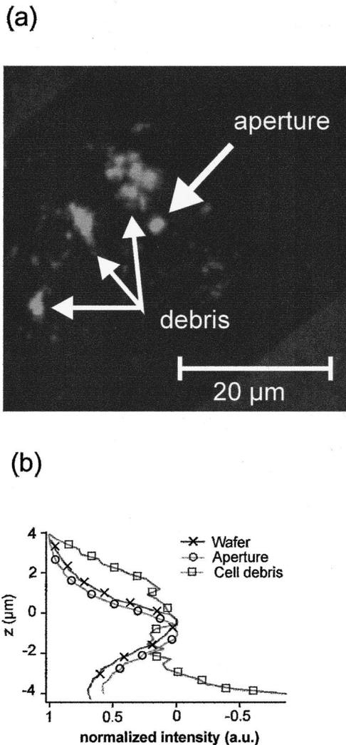
FIG. 3. (a) Fluorescence scanning micrograph taken with a confocal microscope. The cell membrane is labeled with a fluorescent marker (thick arrow). Some cell debris is also visible (thin arrows). (b)  $z$  series taken from the fluorescence of the cell membrane, the  $\text{Si}_3\text{N}_4$  layer, and the debris on top of it.
