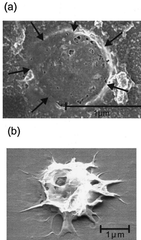
FIG. 2. (a) Top-view of the aperture with incorporated cell material. The arrows indicate the circumference of the opening. (b) Close-up of the cell membrane taken from the backside protruding from the opening.
