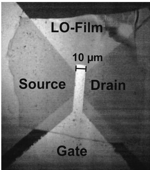
FIG. 3. Micrograph of the realized LO-MOSFET: Pt pads were used for source and drain contacts. The LO film was laterally patterned in order to form a mesa structure in the active region for device isolation.
