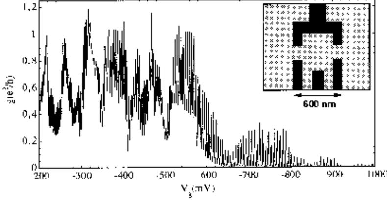
Fig. 1. – Conductance oscillations of a quantum dot in the Coulomb-blockade regime at zero magnetic field as a function of the centre-gate voltage  $V_g$ . Roughly 170 peaks are observed between  $V_g = -200$  mV and  $V_g = -1000$  mV. The inset shows a schematic of the quantum dot. The shaded area denotes the 2DEG and the black areas indicate the gates with which the dot is defined. The lower middle gate is the centre-gate.
