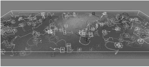
Fig. 5. Example of tracking 160 synthetic spots in a image sequence of 30 100 \times 100 \times 5 image stacks. The various types of simulated dynamics can be appreciated by the variety of the path.
