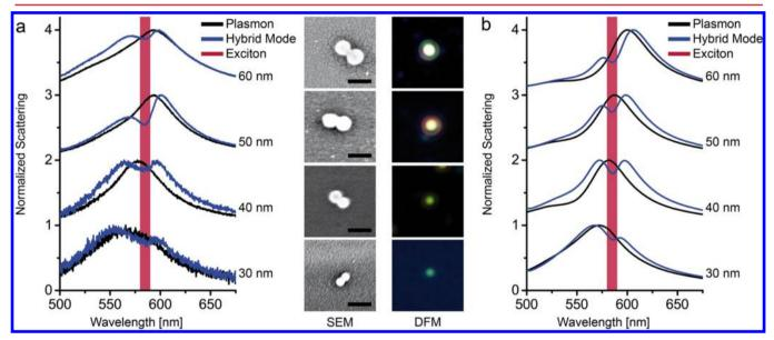
Figure 2. (a) Normalized scattering spectra before (dark-blue) and after (black) photobleaching the J-aggregate for 30, 40, 50, and 60 nm NPs dimers. The spectral region shaded in red covers the energy resonance of the J-aggregate. The right panels show the structures corresponding to each spectrum under SEM and darkfield microscopy. Scale bars: 100 nm. (b) Numerical simulations show excellent agreement with the experimental data.
