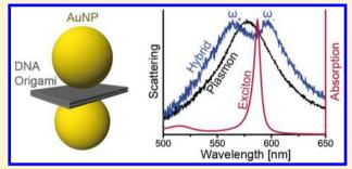
the energy frequency of a J-aggregate exciton. With this system we obtained strong plasmon-exciton coupling and studied farfield scattering at the single-structure level. The individual structures displayed normal mode splitting up to 170 meV. The plasmon tunability and the strong field confinement attained with nanodimers on DNA-origami renders an ideal tool to bottomup assembly plasmon-exciton systems operating at room temperature.
