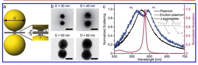
Figure 1. (a) Schematic of a two-layer DNA-origami sheet templating a gold nanoparticle dimer with a designed separation of  $\sim$ 5 nm. (b) TEM images of DNA sheets accommodating NPs of different diameters ranging from 30 to 60 nm. Scale bars are 40 nm. (c) Typical spectra of 40 nm dimer with (dark blue) and without (black) J-aggregates. J-aggregate absorption is depicted in red. Inset shows the chemical structure of the molecular exciton used in this work.
